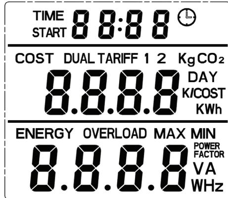
Row 1: Display either the time of day OR the accumulated time for which energy use has been recorded.
