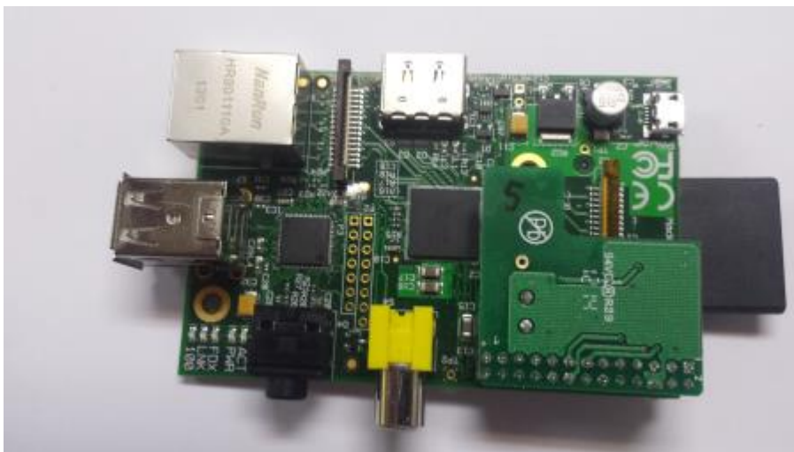
Fig. 1: R-Pi with piggy back RF-transmitter board
