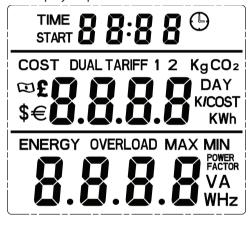
Row 1: Display either the time of day OR the accumulated time for which energy use has been recorded.
