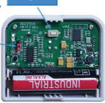
Remove the cover on the compartment of the transmitter using a small coin twisted in the slot between the two halves of the housing and insert the battery - observing the correct polarity.
