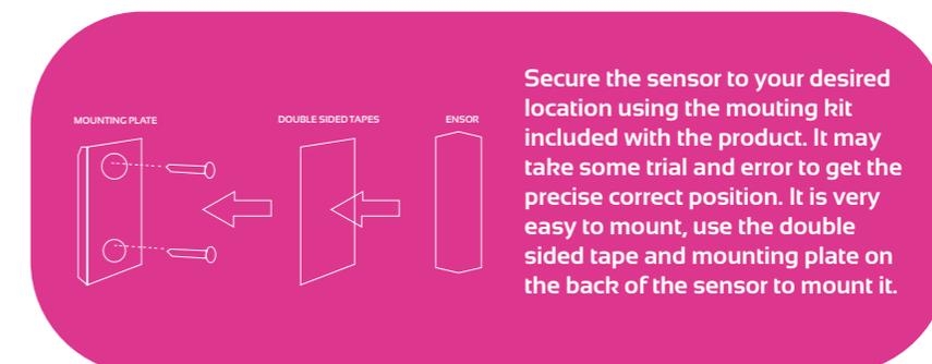
Secure the sensor to your desired location using the mounting kit included with the product. It may take some trial and error to get the precise correct position. It is very easy to mount, use the double sided tape and mounting plate on the back of the sensor to mount it.
