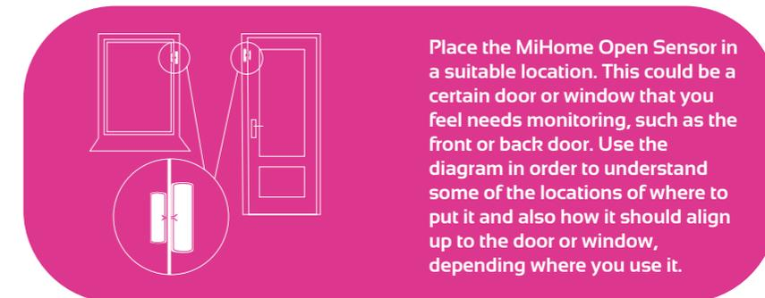
Place the MiHome Open Sensor in a suitable location. This could be a certain door or window that you feel needs monitoring, such as the front or back door. Use the diagram in order to understand some of the locations of where to put it and also how it should align up to the door or window, depending where you use it.
