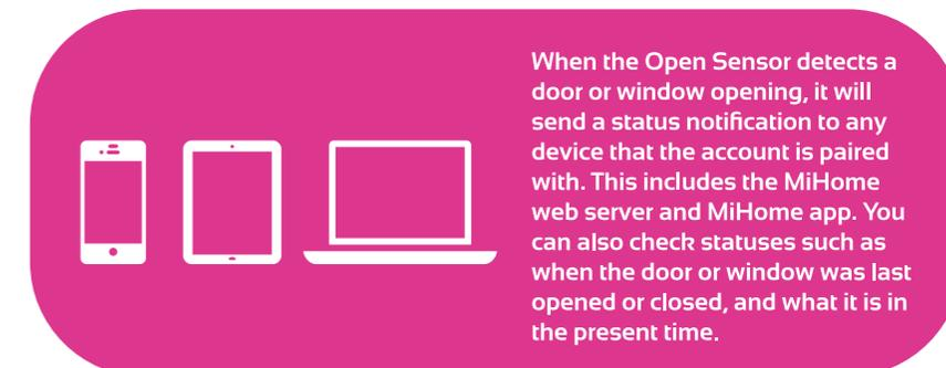
When the Open Sensor detects a door or window opening, it will send a status notification to any device that the account is paired with. This includes the MiHome web server and MiHome app. You can also check statuses such as when the door or window was last opened or closed, and what it is in the present time.
