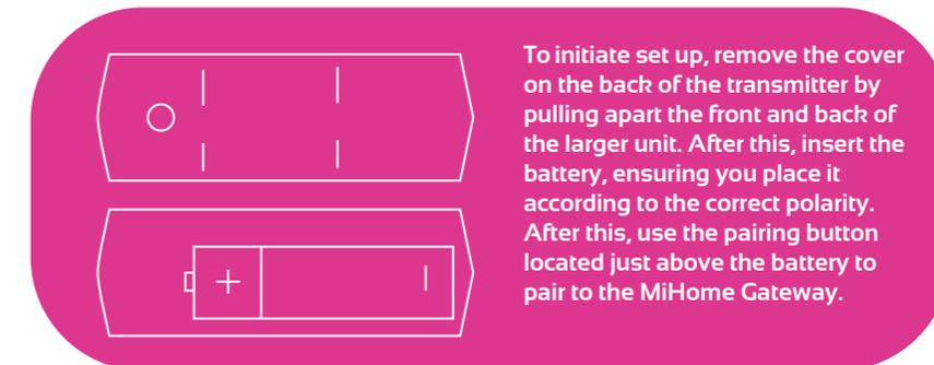
To initiate set up, remove the cover on the back of the transmitter by pulling apart the front and back of the larger unit. After this, insert the battery, ensuring you place it according to the correct polarity. After this, use the pairing button located just above the battery to pair to the MiHome Gateway.
